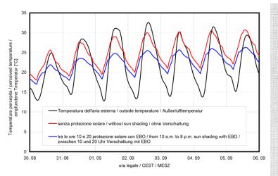
The chart simulates the variation of the indoor temperature of a room as the outdoor temperature changes with and without the use of **Euro Blackout** as a sunscreen.
